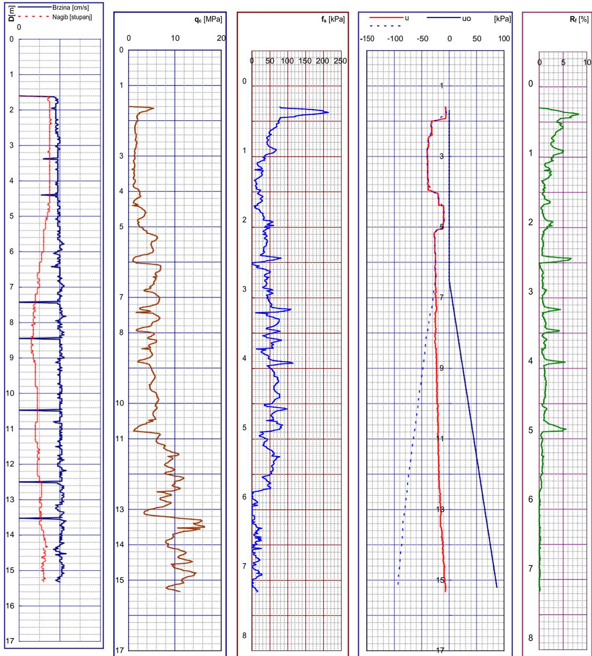
**Figure 3.7** CPTU from thermal powerplant in Sisak, "Blok 3" Čret, (45.4538, 16.4145) (Marić, 2005).
